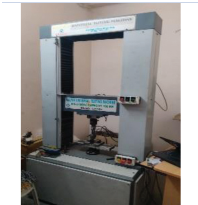
[Table/Fig-5]: Universal testing machine.
